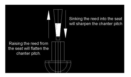
It is important to know that changing the seating of the reed affects the high hand notes more than the low hand notes. For example, if you sink the chanter reed, the High A will sharpen more than the Low A will sharpen. Changing the reed seat is how a piper will get the chanter close to a target pitch, or how a piper will establish the pitch the chanter 'wants' to be at by checking the Low A and High A until they are the desired pitch without any tape.
